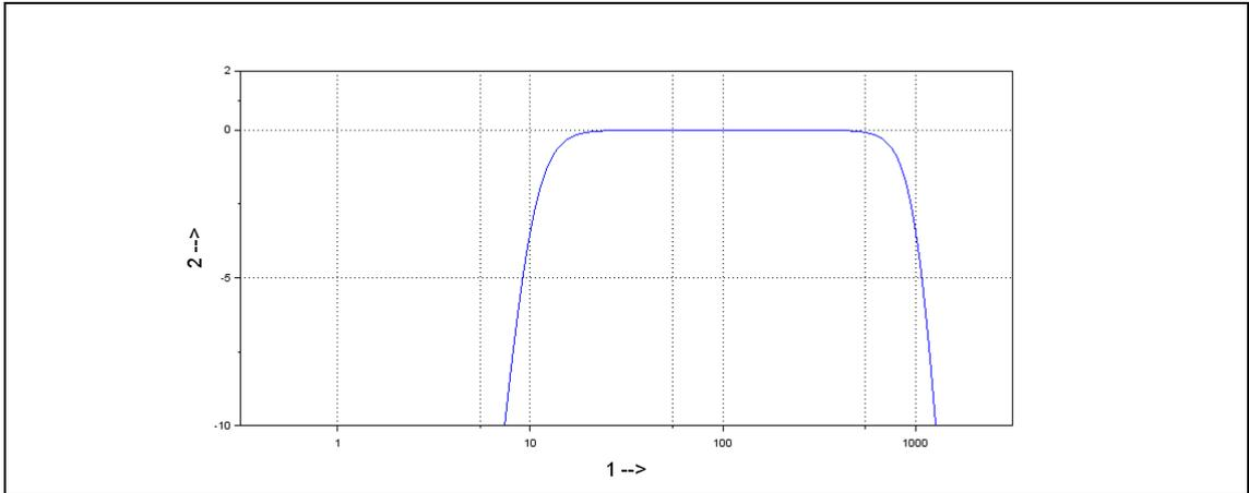
*Fig. 2: Typical frequency response 10 Hz–1000 Hz*
